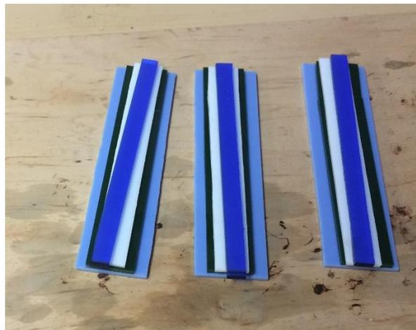
Cut glass stacked, waiting to be glued before fusing
