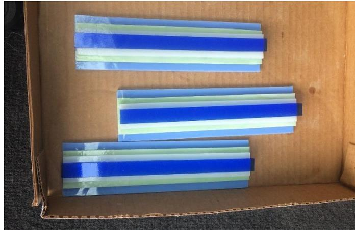
Glass glued together before fusing into a rod
